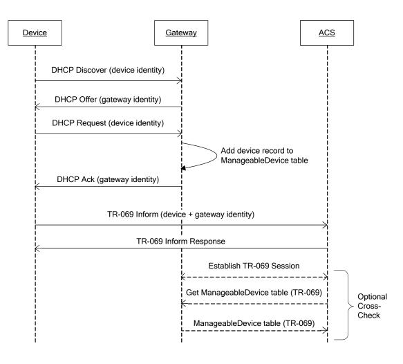
Figure 10 – Device-Gateway Association using DHCP Discover
